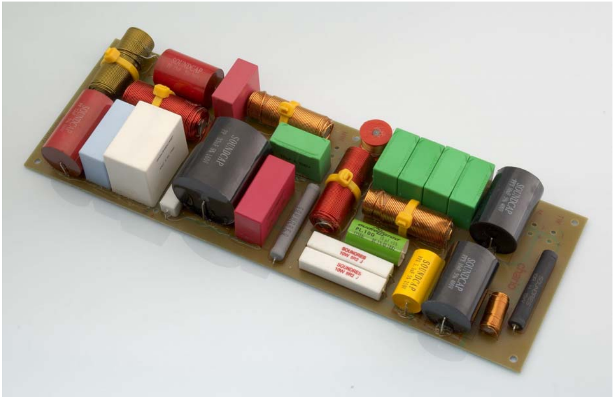
Mid-High Xover – SOUNDCAP™ High Grade Capacitors & MIL Resistors
