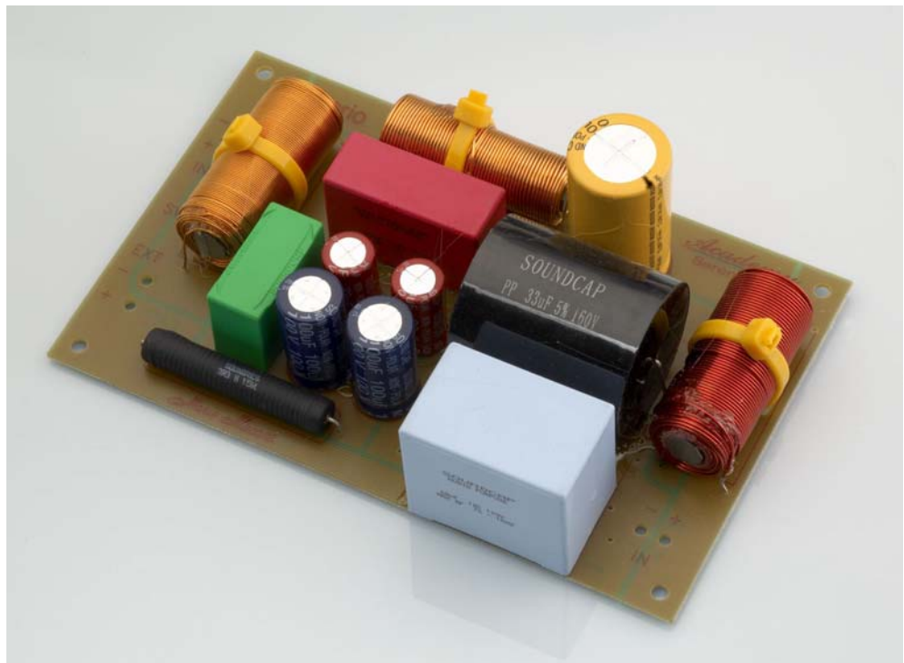
Low Xover – IRON POWDER Cores & HIGH Q Inductors
